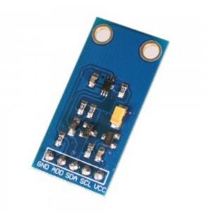
The module I've got measures only 32 x 16mm. I soldered a five pin header onto the PCB and this allowed me to plug it onto a piece of breadboard.
